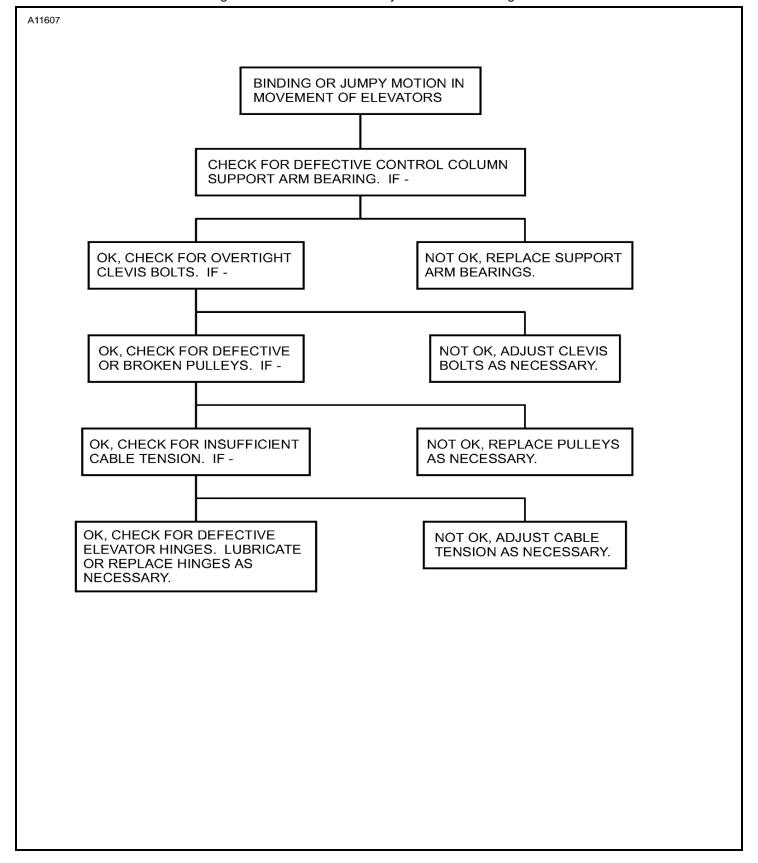
Figure 101: Sheet 1: Elevator System Troubleshooting Chart
